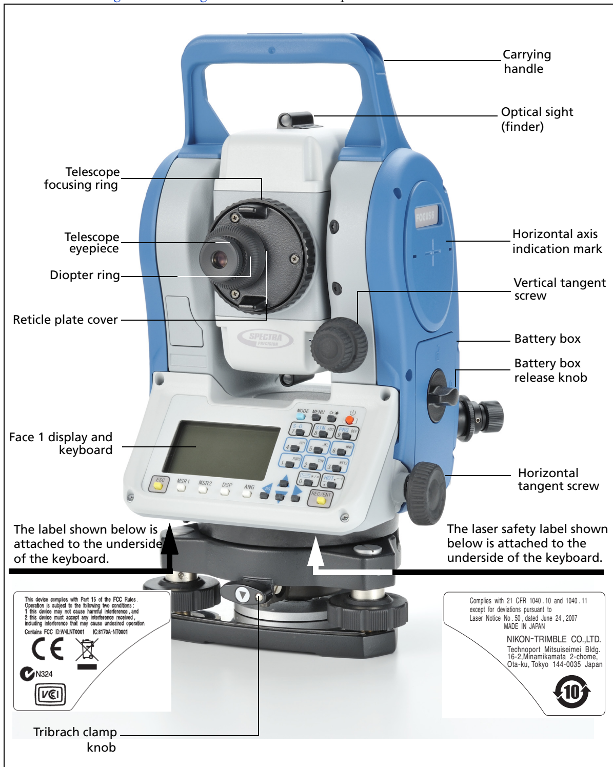
Figure 3.1 Back view of the Focus 6 5" total station (Face 1)
